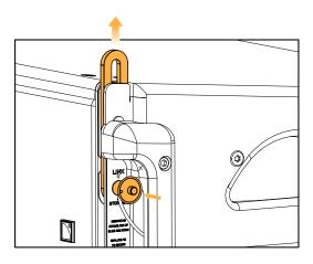
b) Slide up the rear rigging arms and select the same inter-element angle, from 0° to 10°.
