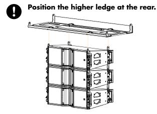
Secure the Kara II rigging arms inside the slits with the ball-locking pins.
