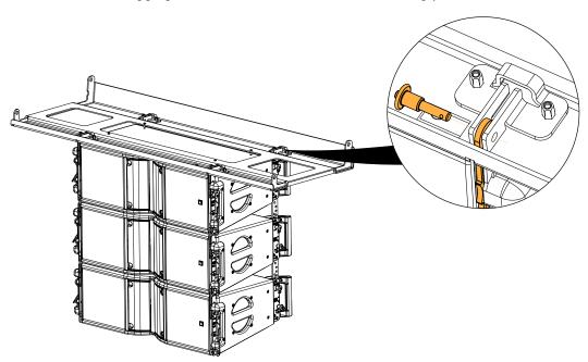
**3.** Lower the K1 array as close as possible to the assembly without resting on it.
