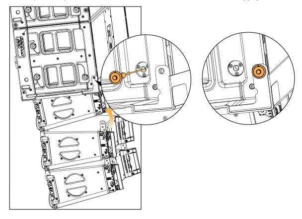
b) Secure the front KARA-DOWNK1 tabs to the K1 rigging. Slightly lower the K1 array if necessary.
